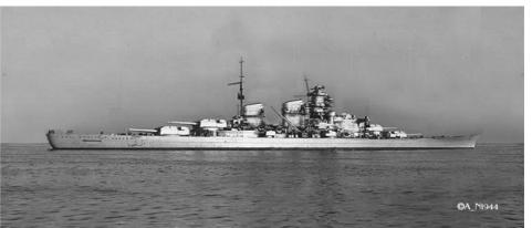
cessors. Designed with a commerce war in mind; diesel engines were selected instead of the usual high pressure steam turbines typically used for ships of this size.
